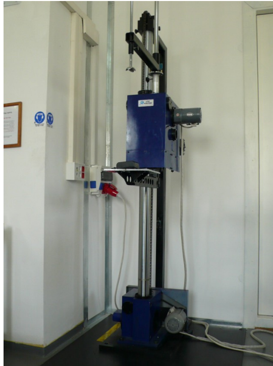
Photograph 6.4.1 Free fall test setup for dropping on face
