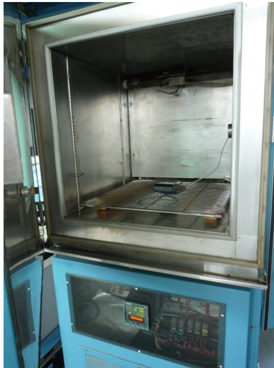
Photograph 6.2.1 The EUT in the low temperature chamber
