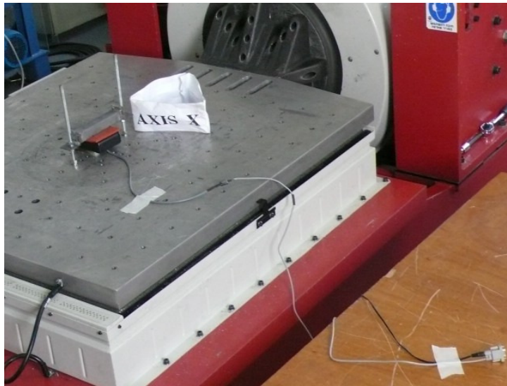
Photograph 6.1.3 Sinusoidal vibration test setup (longitudinal axis)
